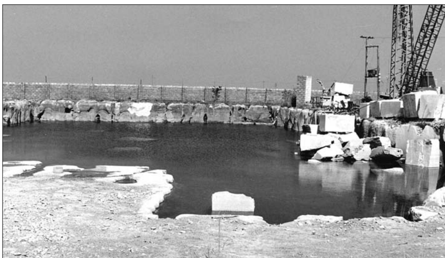
Fig. 3 - Marble quarry East of Lusaka in which the local water table crops out. The excavations expose an intensely karstified marble with solution flutes, rounded karren and phreatic passages in the epikarstic zone.
